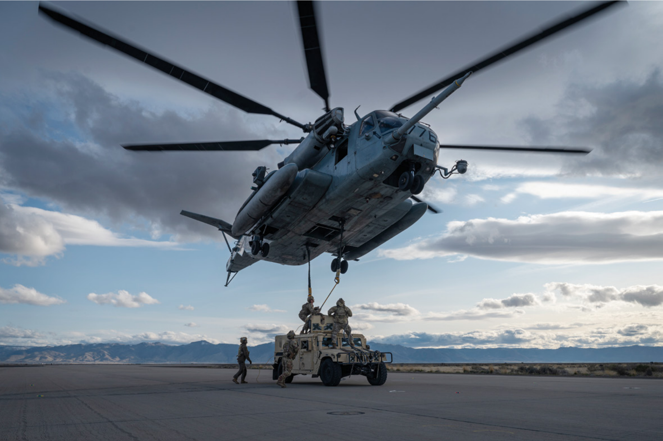
S haring the load: Airmen from the 921st Contingency Response Squadron establish a sling load connection with a CH-53E Super Stallion helicopter from Marine Heavy Helicopter Squadron 361 at Amedee Army Airfield in Herlong, Calif., April 7, 2025. The 921st CRS took part in Exercise Dragon Spark, a 10-day joint training event focused on enhancing rapid deployment capabilities, expeditionary logistics and interoperability between Air Force and Marine Corps units. (U.S. Air Force photo by 1st Lt. Cassidy Fisher) ▲
