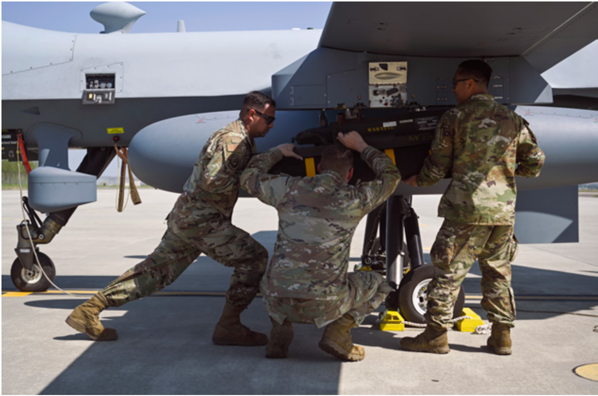
Senior Airman Eduardo Ledezma, left, Tech. Sgt. Kristopher Speir, center, and Tech Sgt. Aldrich Aldana, 163d Attack Wing MQ-9 Reaper armament systems specialists, load an AGM-114 Hellfire missile onto an MQ-9 Reaper at Kunsan Air Base, Republic of Korea, April 30, 2025. The mission-ready platform supports real-time strike options that protect the region’s stability and demonstrate allied resolve in contested environments. (U.S. Air Force photo by Staff Sgt. Daniel Brosam) ▲
